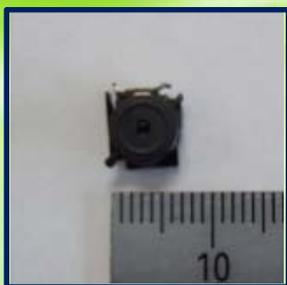
1-mm-diameter mobile-phone camera lens
